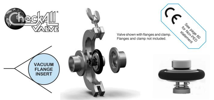
The **Vacuum Flange Insert (VI)** check valve is designed to fit between ISO/NW/KF/QF vacuum flanges designed in accordance with DIN 28403, DIN 28404, ISO 1609, and ISO 2861. It is both a centering ring and a check valve. The compact design requires no additional space in the line. Its size makes it extremely economical when compared to full-bodied valves. The VI valve can also be used as a low pressure relief valve under either positive or vacuum conditions by using the desired spring setting.
