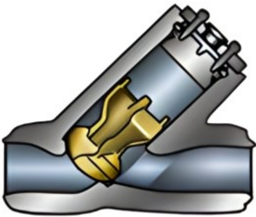
Illustration of inclined, y-pattern poppet style check valve.
