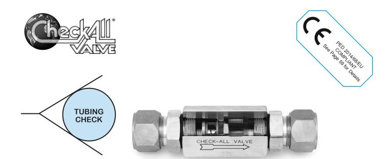
The **Tubing Check (TV)** check valve is constructed with compression tube fittings (flareless) and is designed for a minimum pressure drop. The valves are furnished complete with ferrules and nuts. The TV valve can also be used as a low pressure relief valve or vacuum breaker by using the desired spring settings.
