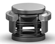
The Straight Sided Insert (SI) is a threadless check valve designed to be inserted into any cavity where a check valve is needed and threads are not desired. Consult the factory if your application requires tolerancing for a press fit installation. The SI valve can also be used as a low pressure relief valve or vacuum breaker by using the desired spring settings.
