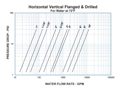
**Note:** All flow curves and Cv values presume the valves are fully open with 1/2 PSI cracking pressure springs.
