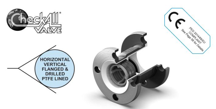
The Check-All® Flanged & Drilled — Fluoropolymer (PTFE) Lined (HT) check valve is a one piece body with ANSI/ASME B16.5 Class 150 flanged ends. The valve has a solid one piece PTFE liner which covers the flange faces out to the raised face diameter. All wetted surfaces are fluoropolymer (PTFE/FEP/PFA) including the FEP encapsulated stainless steel spring.
