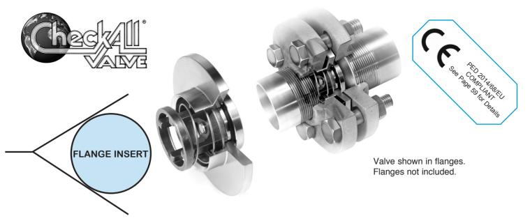
The **Flange Insert (F1, F6, FP)** check valves are the ultimate valves in flanged systems. They provide the simplest and most economical way to install check valves in a piping system. The valve body helps position itself while bolts are being installed and tightened. Two gaskets are required instead of the one normally used in a flanged joint. See page 55 or consult the factory for additional installation guidelines.
