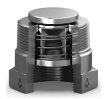
The **Bushing (BU, BR)** check valve is a valve with a standard bushing housing. This valve is adaptable to many types of service applications. It has very little restriction and produces a low pressure drop. It can be used quite effectively in systems where flow and pressure drop are critical by the use of a reducer coupling. The BU valve can also be used as a low pressure relief valve or vacuum breaker by using the desired spring settings.
